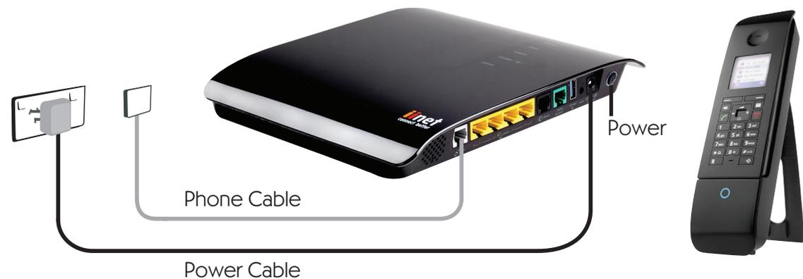
1. Connect the power adapter to the power port on BoB2™. Plug the power adapter into the wall socket. Turn the BoB2™ power button on and wait for the green light to illuminate.
