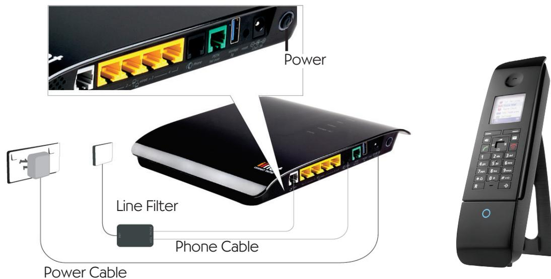
1. Connect the power adapter to the power port on BoB2™. Plug the power adapter into the wall socket. Turn the BoB2™ power button on and wait for the green light to illuminate.
