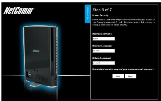
Figure 6: Setup Wizard Step 6 - Router Security Settings
