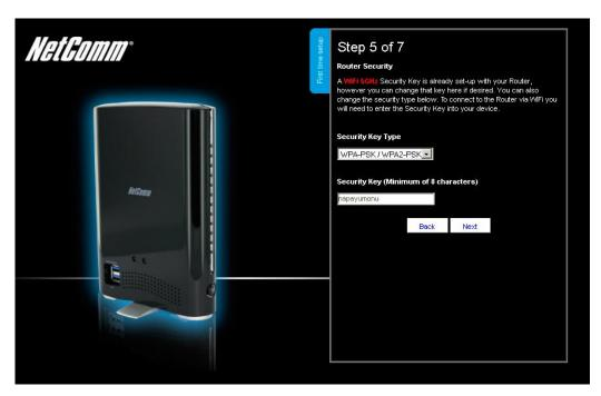
Figure 5: Setup Wizard Step 5 - 5.0 GHz Wireless Security Setup
