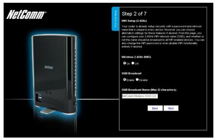
Figure 3: Setup Wizard Step 2 - 2.4 GHz WiFi Setup
