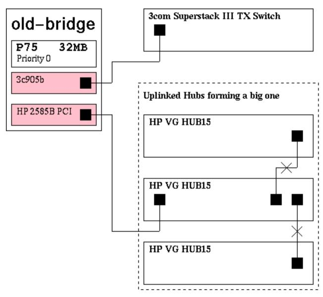
Figure 1. Hardware setup Of The Old Bridge Scenario
